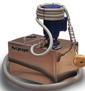
The Natgraph Solvent Recirculation Unit is made of stainless steel, consisting of a 30 litre, freestanding holding tank that contains a filter basket, and flameproof solvent pump which complies with the ATEX directive 94/9/EC, required by European legislation for electrical and mechanical equipment used in potentially explosive atmospheres.
