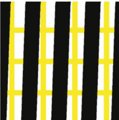
special surface treatment, sometimes it's to do with the precise geometries of the two meshes. Depending on how squashed (or calendared) the two meshes are, the ink-in-the-mesh-at-the-start will be slightly different. That's one reason (amongst many) why it's a scandal that mesh manufacturers don't provide this figure. If you don't know in advance how much ink is in there then your second task – knowing how much remains – is even harder.
