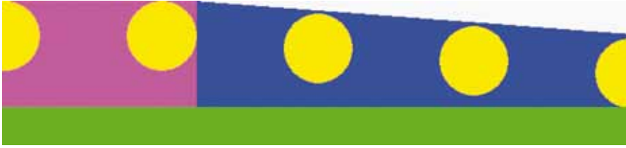
The ink is thicker at the edge because of the EOM, but normal in the middle ...
