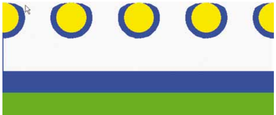
Ink deposit = Ink-in-the-mesh-at-the-start minus Ink-on-the-mesh-at-the-end
