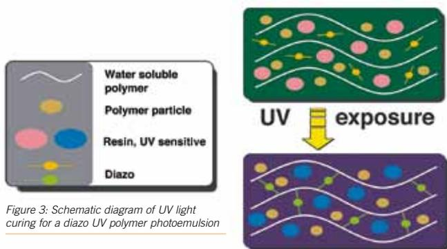
Figure 3: Schematic diagram of UV light curing for a diazo UV polymer photoemulsion
