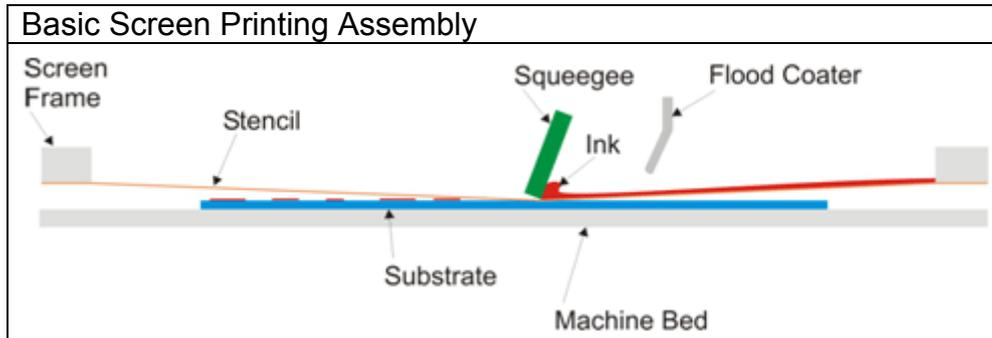
The importance of the flood coater is not recognised and is treated as a spreader. It should be that is given as much consideration as the squeegee.
