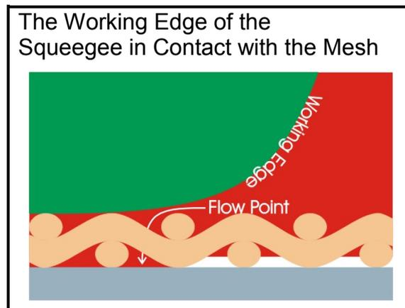
As the squeegee moves through the ink across the top of the stencil, it creates a wave in the ink. Within this wave, the ink is circulating with the bulk of ink rolling in front of the squeegee across the stencil.
