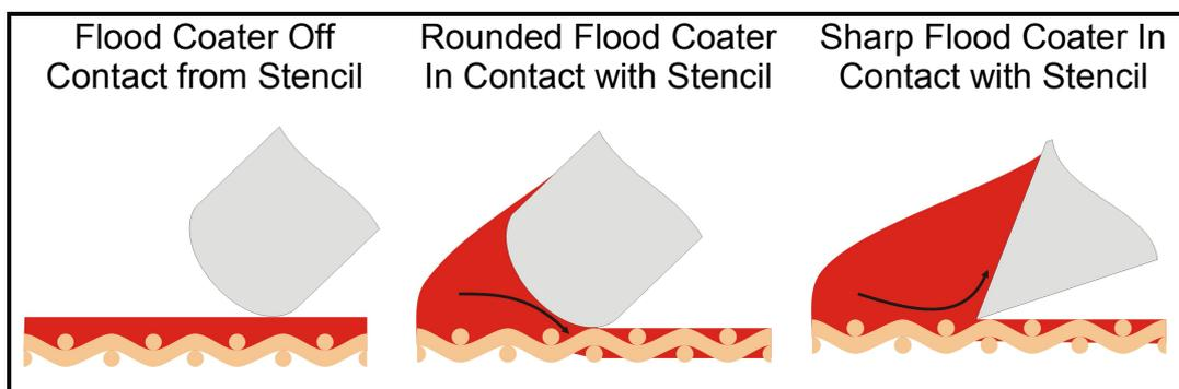
The graphic demonstrates with the coater off contact mesh charging is minimal. The rounded profile charges the mesh more than the sharp profile. Generally printers tend to use a rounded edge for large solid areas and the sharp edge for four-colour process work. If the ink is opaque then the condition of the flood coater is not so important because the effect is not visible. However if the image is a halftone or the ink transparent then faults in the flood coater are very apparent.
