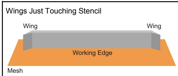
The flood coater with wings has to be machined very accurately as the bottom of the wings needs to touch the stencil but not damage it.
