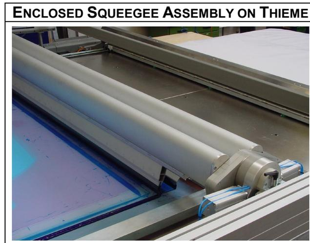
The squeegee mechanism, so often a headache on large format machines is built like a brick outhouse. Hefty but not crude the mechanism has very fine adjustment and balanced pressure along its length. It is easy for one person to unload and load the squeegee carrier.
